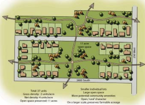
The top graphic depicts a traditional approach to residential development, with individual lots comprising all of the space. The lower graphic shows an open space design approach to the same development, which maintains over 50% of the space as open space.
